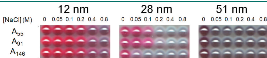
Figure 4. Optical photographs illustrating the effect of increasing salt concentration on the aggregation behavior of selected polymer-coated gold nanoparticles. The images show small sections of 96-well plates containing nanoparticles in NaCl solutions, following 1 h incubation at room temperature.
